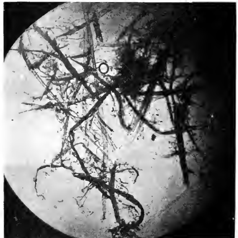
Mixture of 25 per cent Sulphite and 75 per cent ground wood, by weight.
